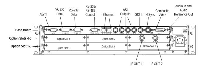
Figure 1.13: E5750 (2U) Rear Panel Component Parts and Connectors
